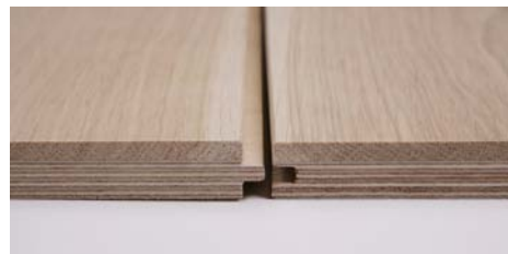
Multilayer product. 5.7mm top layer on 12mm (or 9mm) plywood core
